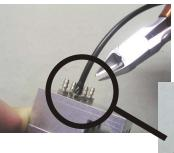
With a side-cutter the hose is cut beside the connection-nipple
